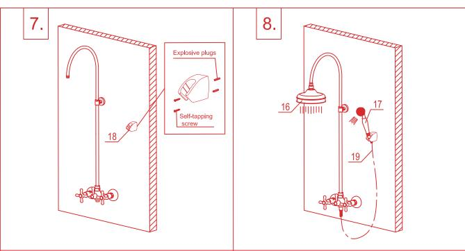
7.With utilizing location of shower hook(18),to drill hole of 2-Ø6 on the wall properly. To fasten Shower hook on the wall of reserve location with utilizing the self-tapping screw & explosive plugs in the Shower hook.
