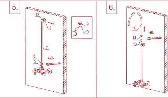
5.First cover the installation seat with the decorative cover2 (8), then, insert the Medium-section pipe(7) into Cone o'ring (5)and Nut 1(6),assemble with Main body & installation seat. Atter adjust position properly,use screw-driver to tighten the Self-tapping screw(9). Adjust decorative cover 2 to the wall at the same levelby hand. Then, use allen key to fasten Medium-section pipe throughScrew(12). At last, use spanner to fasten Nut 1 on Medium-section pipe;
